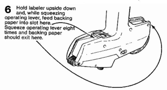
If backing paper does not become taut and exit at rear: Turn labeler upside down, squeeze operating lever and pull backing paper out of slot. Repeat steps 4, 5, and 6.
